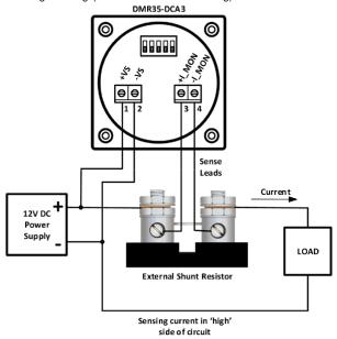
It is also possible to use the meter to monitor voltage in a circuit that is independent of the meter's power supply circuit, as shown in the schematic below. When used in this way, the meter's current measuring terminals may electrically float with respect to its power supply terminals, as long as the voltage difference between the two terminal pairs remains within +/- 48V of each other.
