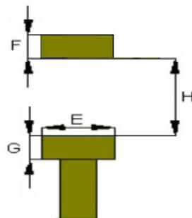
This is the feed-line to the Antenna and should be matched to 50 Ohms based upon the PCB dielectric parameters.
