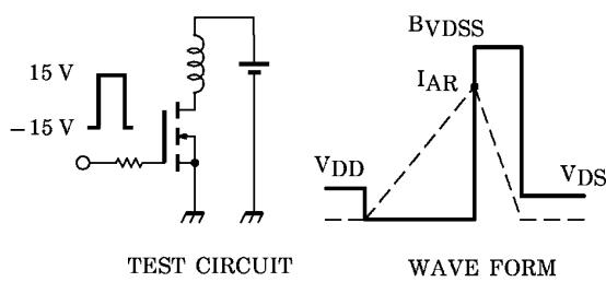
$$R_G = 25 \Omega \quad EAS = \frac{1}{2} \cdot L \cdot I^2 \cdot \left( \frac{B_{VDSS}}{B_{VDSS} - V_{DD}} \right)$$
