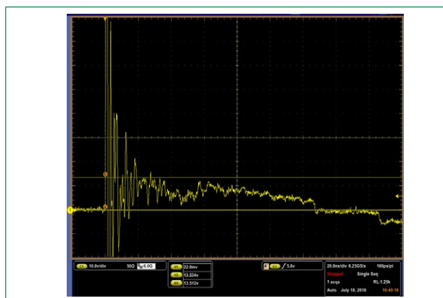
IEC 61000-4-2 +8 kV Contact ESD Clamping Voltage
