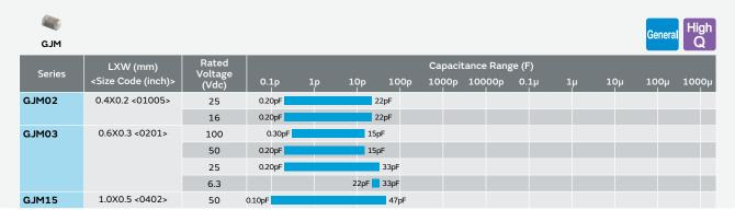
■ High Q Chip Multilayer Ceramic Capacitors for General Purpose (>100Vdc)
