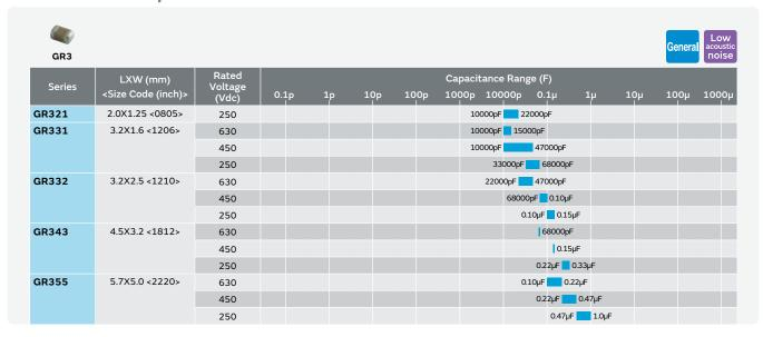
Chip Multilayer Ceramic Capacitors with Soft Termination for General Purpose
