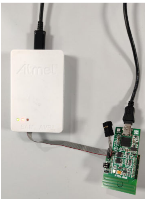
Figure 4-11. Connecting Programmer/Debugger with ATSAMR30M Sensor Board
