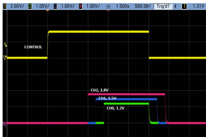
Figure 6. Sequencing Output Channels with DC2028A Using TON_DELAY and TOFF_DELAY
