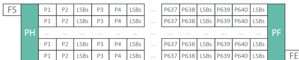
Figure 20: Example of pixel ordering for one full frame transmission
