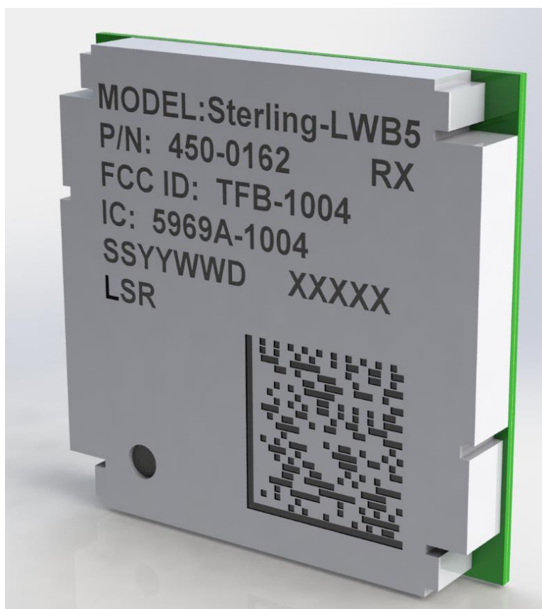
Figure 1 Sterling-LWB5 Base SIP Module (450-0162)
