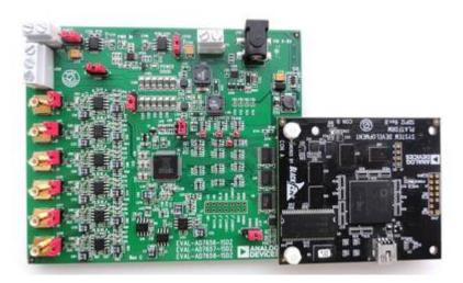
The **EVAL-AD7658-1SDZ** evaluation board is a member of a growing number of boards available for the **SDP**. It was designed to help customers evaluate performance or quickly prototype new **AD7658-1** circuits and reduce design time.
