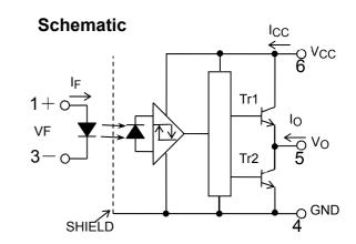
0.1 μF bypass capacitor must be connected between pins 6 and 4.
