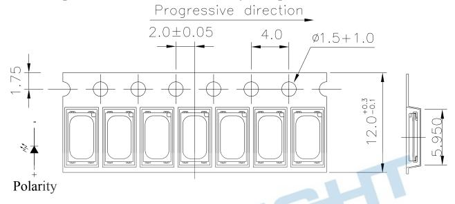
**Note:** 1. The tolerance unless mentioned is  $\pm 0.1$ , unit = mm.
