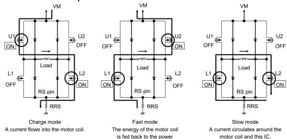
**Operation Function of Output Transistor**
