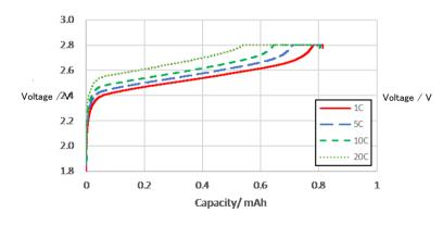
Charge : CC-CV 1C, 2.8V, cut-off 0.05C at 25°C
