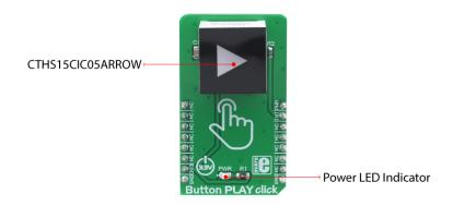
The arrow icon on the top of the touch sensor is visible even when the backlight is off, thanks to the LEXAN™ polycarbonate film with an inverse print of the icon, placed on a top of the sensor. When the internal LEDs are turned ON, the light will pass through the translucent arrow icon, resulting in a uniformly lit arrow icon. An interesting lighting effect can be designed when touched, by applying a PWM signal to the IN pin.
