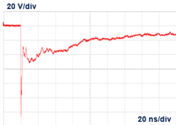
Figure 6. ESD response to IEC 61000-4-2 - C = 150 pF, R = 330 Ω (-8 kV contact discharge)
