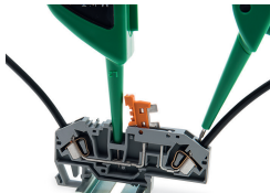
Testing via jumper contact slot.
