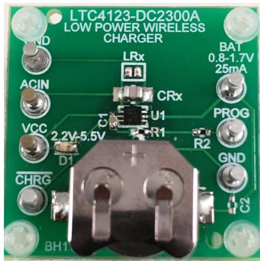
Figure 1. Demonstration Kit with Battery
