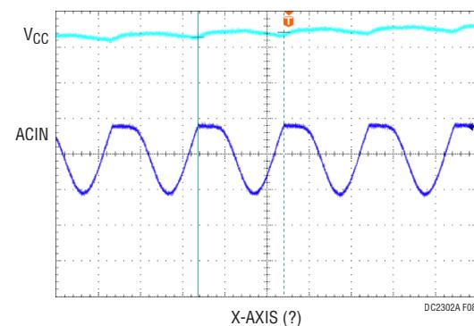
Figure 9. DC2300A  $V_{IN} = 5\text{V}$ , Air Gap = 4mm
