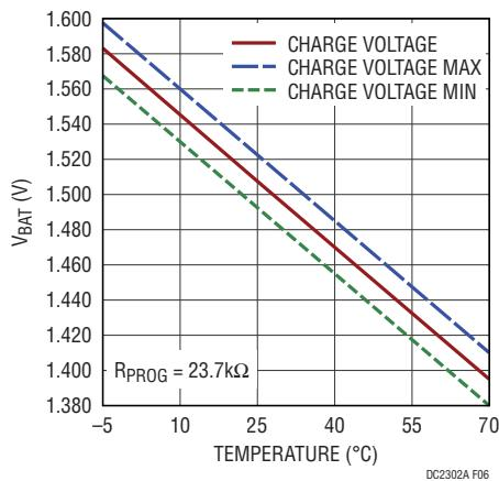
Figure 7. Charge Voltage vs Temperature (Placeholder)
