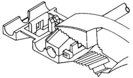
Close cover, keep wire in position and squeeze with pliers until cover is locked.
