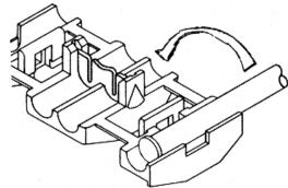
Insert wire in cover. For installation of two through wires, remove wire stop.
